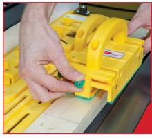
3. For narrow pieces, such as table legs, the outside leg of your GRR-RIPPER may hang out beyond the edge of the workpiece. In this case, add the GRR-RIPPER's Adjustable Spacer along with a user-made riser block for extra support. Riser block size and dimension will vary depending on the dimensions of your workpiece. Press down firmly on the GRR-RIPPER.
