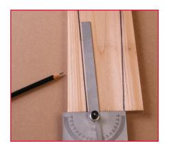
2. To set the scale, lift up on the adjustment knob and pivot it. For whole and half degrees, use the pointer marked with the red 0.
