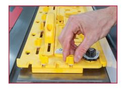
2. Unbolt the Top Plate from the Pivot and Locking Knobs. Shift 1" forward and reattach it through the two Jointing Slots. In this position the Top Plate can slide laterally to accommodate wider boards.
