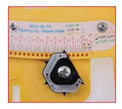
**3.** Use the green lines along with the pointer marked with green numbers for 1/8° and 5/8° (.125° and .625°) angles. Here the jig is set for 3 1/8° (3.125°). As long as you follow the COLORMATCH, it is nearly impossible to go wrong.
