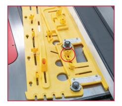
The MICRODIAL Tapering Jig may be used as a large pushblock to straighten the edge of crooked boards on your tablesaw. Attach the Trailing Block and shift the jig's Top Plate to the Jointing Slots. The MICRODIAL Tapering Jig can straighten the edges of boards up to approximately 12" wide and 30" long.
