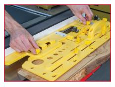
**3.** To make the cut, hold the jig on top of your workpiece with the Trailing Block hooked on the trailing end of the board. Guide the jig along the fence, pushing the board as you go. For even more support, add one or two GRR- RIPPER GR-200s.
