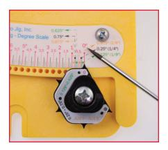
2. Repeat the process at the other end of the scale aligning red 10° line with the same 0° pointer. Tighten the screws and double check to make sure nothing shifted. Your jig should now be calibrated. Use the same technique to calibrate the rise and run scale.
