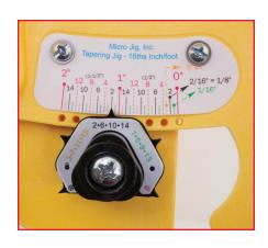
**4.** For the sixteenths, use either the pointer near the yellow or green numbers aligned with the yellow or green lines respectively. Here the jig is set to cut a taper of 1 3/16" per foot.
