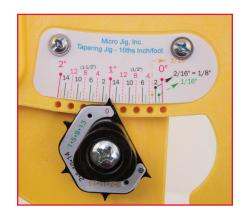
3. To set the jig for the 1/8" inch divisions (1/8", 3/8", 5/8", 7/8"), align the pointer near the black numbers with the appropriate black line on the scale. Here the jig is set to cut a taper of 1 1/8" per foot.
