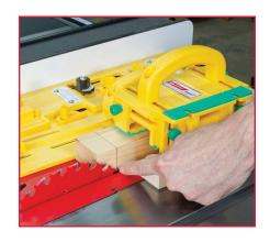
4 sides of the leg then tilt the saw blade to 45-degrees and reset the jig to the desired rise and run or degree. Notice the bigger the angle will result in a steeper taper cut. Use your best judgment on the style and design of your tapers. In the example image, the piece tapers to an octagon at the bottom, so the setting was 3 times the original taper of 3/4" per foot. Reset the fence to have the taper start in the desired place.
