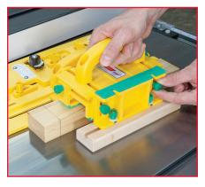
Tighten the knobs to ensure the GRR-RIPPER has good traction.
