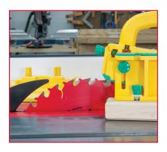
2. At the trailing end, the blade is significantly above the stock surface and just barely clears the underside of the GRR-RIPPER. In this case, shifting the GRR-RIPPER forward provides just enough clearance for a safe cut.
