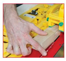
4. Make the tapers as usual, rotating the piece clockwise after each cut. NOTE: if you are using a right-tilt saw, Pay close attention to where the blade is as you will be cutting along the upper corner of the workpiece.
