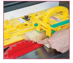
saw blade no more than 1/4" (.25") above the surface of the workpiece. Ensure that the saw blade passes through the GRR-RIPPER tunnel.
